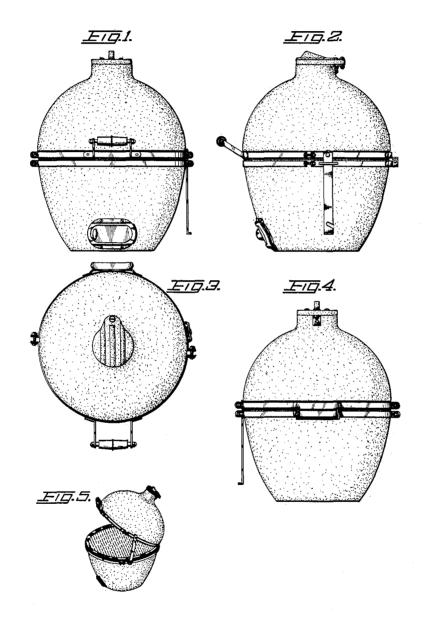
FIGURE 1 is a front elevational view of a combined barbecue grill and smoker, showing my new design;
