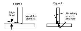
The welding engineer should also check the welding electrodes which are being used for high silicon levels. Excessive silicon can cause zinc to penetrate the weld metal, leading to cracking, especially when the zinc coating is thick. The silicon in welding electrodes should not exceed 0.85%; this means that commonly used ER70S-6 filler metals should not be used when welding galvanized steel.
